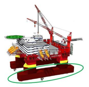
Figure 2: Pontoons of the Vessel (circled in green)
